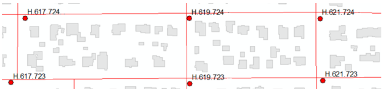
Figure 16: Hydrants showing variations of precision and delimiter in the asset name.
