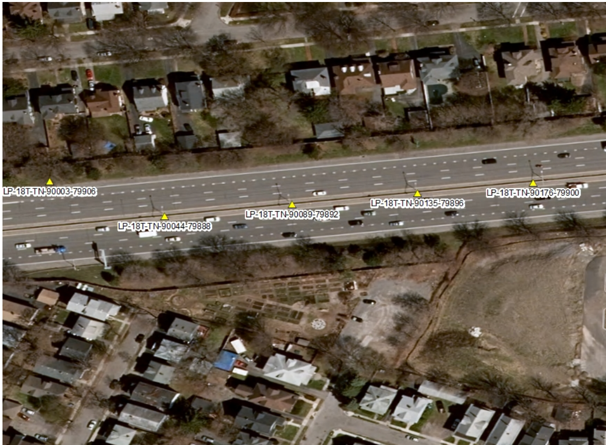
Figure 3: Sample of asset naming: light poles along a highway in New York. Photo courtesy of Mary Susan Knauss.
