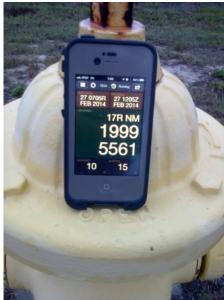
Figure 1: Hydrant and smartphone showing full USNG coordinate associated with an asset near Titusville, Florida. Photo courtesy of Al Studt.
