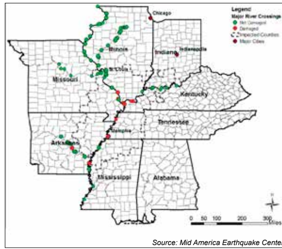
Figure 5-4: Major Damage to River Crossing Bridges in NMSZ
