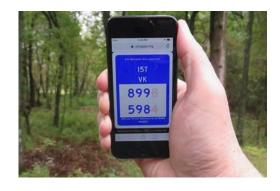
The USNG uses a string of up to 15 characters to describe a location. The first three characters are a **GRID ZONE** designation. Next, two letters identify a **100,000 meter SQUARE** (100 km, about 62 miles square) in the **GRID ZONE**. Then come distances in meters (m) from the **100 km SQUARE's** lower left corner, **RIGHT** (**Easting**), **THEN UP** (**Northing**)!
